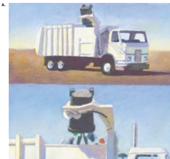
A. HEIL ENVIRONMENTAL'S UNIQUE FORMULA 7000 SPLIT BODY AUTOMATICALLY COLLECTS REFUSE AND CO-MINGLED RECYCLABLES AT THE SAME TIME.
